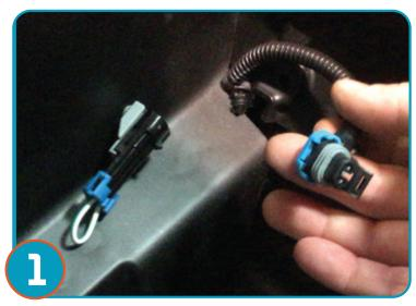
After removing seats from vehicle and removing the OEM seatbelts. Your last step in removing the seat belts will be to unplug the OEM Belt plug by simply unlugging.
