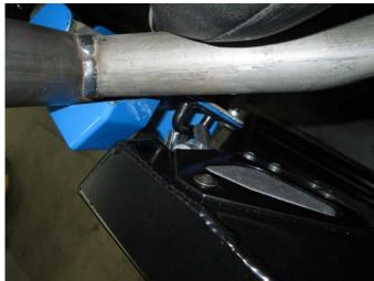
15. Next, adjust the position of the paddle latch, either by sliding it forward or back, until you can open and close the door smoothly. The paddle latch should engage and disengage the door latch catch with no binding. Once you are satisfied, tighten the 3 M6 button head flanged bolts with a 4mm Allen.
