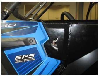
9. Adjust the position of the door so that the lines of the paddle latch housing follow the lines of the plastic trim on the vehicle. Once you are satisfied, tighten the T40 Torx bolts. It may be helpful to have someone hold the position of the door while you tighten the T40 Torx bolts.
