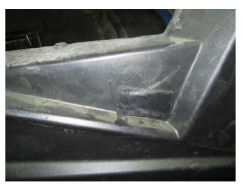
11. Lastly, place one of the adhesive rubber strips supplied in the hardware kit on the front lower corner of the rocker panel. This will eliminate any rattle between the door and plastic.
