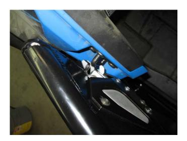
10. Next, adjust the position of the paddle latch, either by sliding it forward or back, until you can open and close the door smoothly. The paddle latch should engage and disengage the door latch catch with no binding. Once you are satisfied, tighten the 3 M6 button head flanged bolts with a 4mm Allen.
