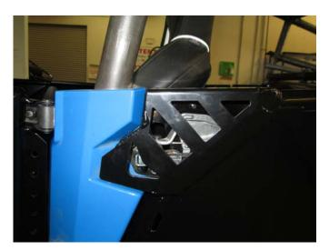
14. Adjust the position of the door so that the lines of the paddle latch housing follow the lines of the plastic trim on the vehicle. Once you are satisfied with the positioning of the door, tighten the M8 bolt and nut on the lower mounting bracket with a 13mm socket and wrench. Then, tighten the two M10 bolts and nuts on the upper mounting bracket with a 15mm socket and wrench. It may be helpful to have someone hold the position of the door while you tighten all of the hardware.
