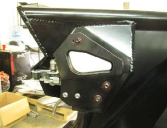
7. You will now attach the latch plate with paddle latch to the door frame. Use 3 of the M6 button head flanged bolts supplied in the hardware kit to attach the latch plate assembly to its corresponding door frame. Front doors are pictured above, while rear doors are pictured below. Leave the hardware hand tight so that you can adjust the position of the latch later.
