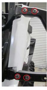
1. Remove front doors by unfastening the 4 T40 Torx bolts holding the door to the upper and lower hinges. Retain all hardware.
