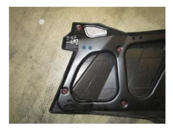
3. You will now need to remove the paddle latch from the stock doors. To do this, remove the 4 T25 Torx screws (circled in red) and the 2 T30 Torx bolts (circled in blue). Retain the T30 Torx bolts; you will use them to install the paddle latches onto the Proarmor doors. The front door is pictured on the left and the rear door is pictured on the right.
