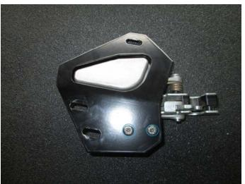
6. Use the 2 T30 Torx bolts you removed earlier to attach the paddle latch to the latch plate.
