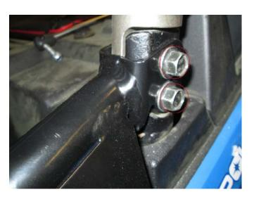
13. Slide the upper mounting bracket over the cage connectors as shown. Reinstall the 2 M10 bolts and nuts you removed earlier. Leave hand tight.
