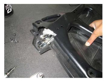
4. Then, pull the steel frame away from the plastic outer shell and remove the latch from the door.
