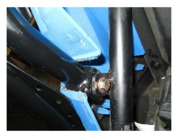
12. Take the rear door and slide the lower mounting bracket through the opening in the plastic. Make sure the bracket sits on the outside of the mounting tab on the chassis. Fasten using 1 M8 bolt and 1 M8 nut, supplied in the hardware kit. Leave hand tight.
