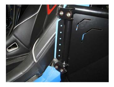
8. Install the front doors using the 4 T40 Torx bolts removed earlier. Leave hand tight so you can adjust the position of the door.
