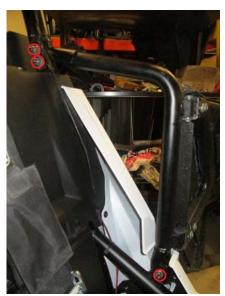
2. Remove rear doors by unfastening the 2 M10 bolts and nuts holding the upper mounting bracket to the cage connector using a 15mm socket and wrench. Retain this hardware. Then remove the M8 bolt from the lower mounting bracket using a 13mm socket. You will not use this bolt for the Proarmor door install.
