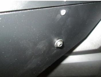
12. Loosely install half clamps to the quarter panel using the provided M6 bolts. Line the quarter panel with the door frame, making sure the edges of the quarter panel run along the center lines of the tube. Tighten down hardware. This concludes the quarter panel install.
