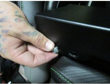
11. Locate the rear lower mounting hole on the stealth door skin. You will need to drill a hole through the stock door plastic using a drill and 1/4" drill bit at this location. Once this is done, secure the door to the plastic using the provided M6 bolt, washer, and acorn nut. Repeat this for the front lower mounting hole. This concludes the rear door install.
