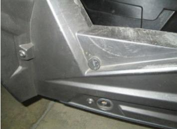
6. Finally, using a drill and 1/2" drill bit, drill a hole into the front lower corner of the door area on the plastic. Once this is done, insert the provided push-in bumper. This concludes the front door install.
