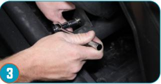
Now you can remove the seat from the car and begin to take the 2 seat sliders out. First remove the bolts on the front of each seat slider with a 13mm wrench and socket.
