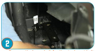
Remove the lower bolt for the stock seat belt with a 16mm socket or wrench.
