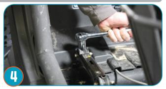
Then remove the 2 nuts from the back of the seat sliders with an 18mm socket.
