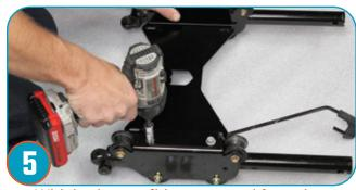
With both seat sliders removed from the car place your new pro armor seat base on and align with the 4 bolts. Re-use the stock bolts that were removed in step 1. Use a 13mm socket.
