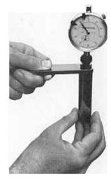
With the gauge positioned so the extension is inside the calibrating tube, slide the dial indicator into the collet until the needle reads zero, then tighten the collet.
