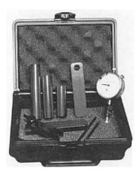
The Universal Pinion Depth Setting Tool may be used to measure pinion depth of most automotive and truck differentials. Measurements are obtained by attaching the tool to the machined bearing cap mating surface in the housing and checking the distance to the pinion gear. Three dial indicator extensions (2", 3" and 4") are included to accommodate a variety of rear end types.
