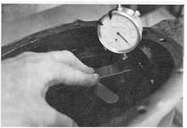
5 - Install the appropriate extension, calibrate the dial indicator to zero, then check to make sure the machined cap surface is square with the pinion. Measure pinion depth with the extension contacting the pinion at a point close to the end of the housing on which the tool is mounted. Reposition the indicator so it contacts the pinion about an
