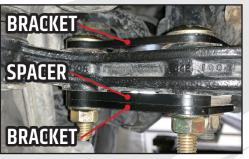
When installing the JL Nexus EF Steering Stabilizer with the TERAFLEX JL HD Forged Front Adjustable Track Bar it is possible for the JL Nexus EF Steering Stabilizer to make slight contact with the Track Bar's joint housing. Installing the tie rod bracket spacer **BELOW** the tie rod instead of above will eliminate this possibility.
