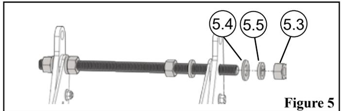
6. Tighten inner nuts (5.3) and lock washers (5.5) outward against gusset (2) shown in **Figure 5**
