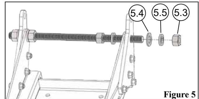
6. Tighten inner nuts (5.3) and lock washers (5.5) outward against gusset (2) shown in **Figure 5**
