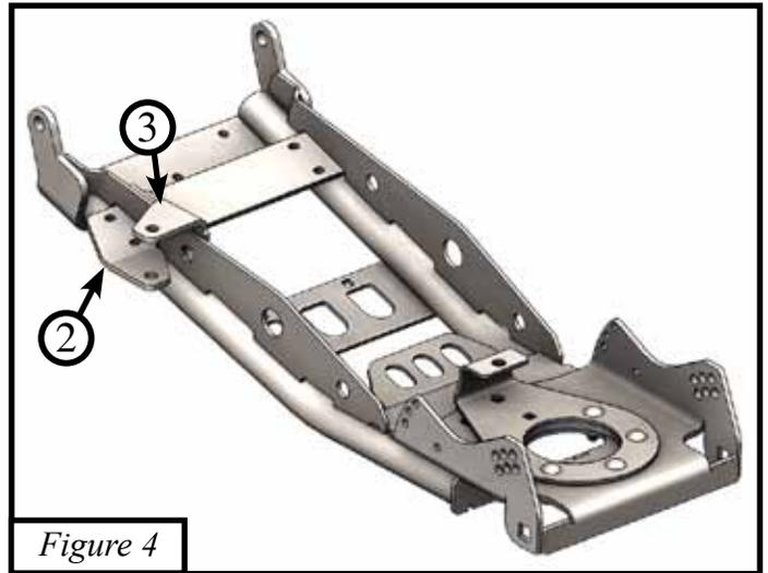
4. Insert the four U-bolts (5.3) through the rear brackets (2 & 3) shown in *Figure 5*. Loosely attach the 5/16" nuts (5.2) to the U-bolts.
