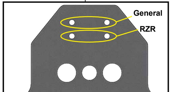
"Figure 3" Mount plate Install
