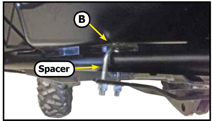
*"Figure 5" Spacer Install*
