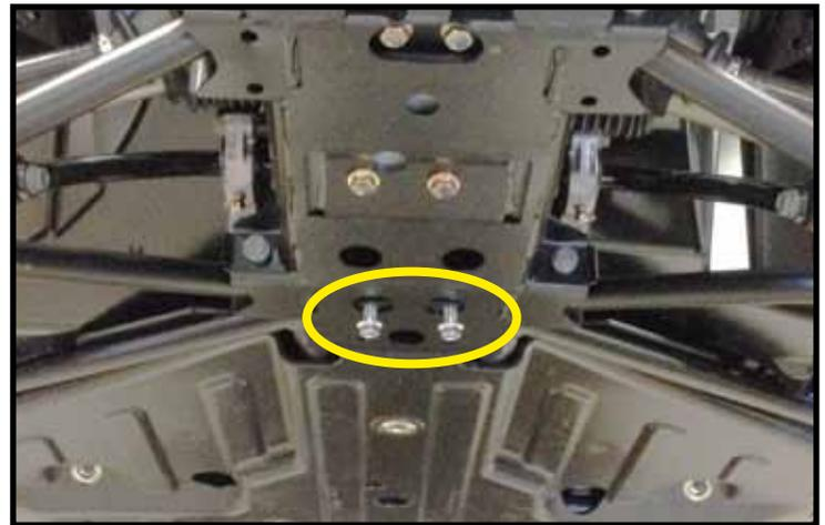
"Figure 2" Bolt Plate Install Location
