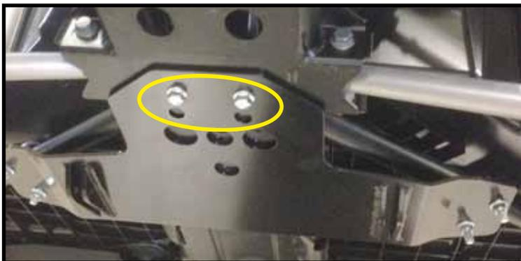
"Figure 4" Mount Plate Install
