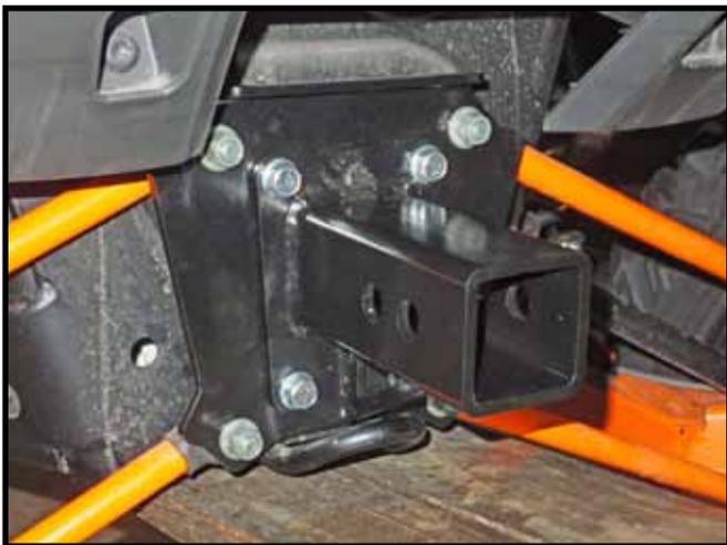
"Figure 5" Receiver Install
