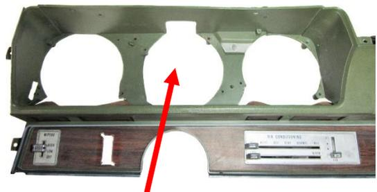
Stock Bezel and Gauges Removed
