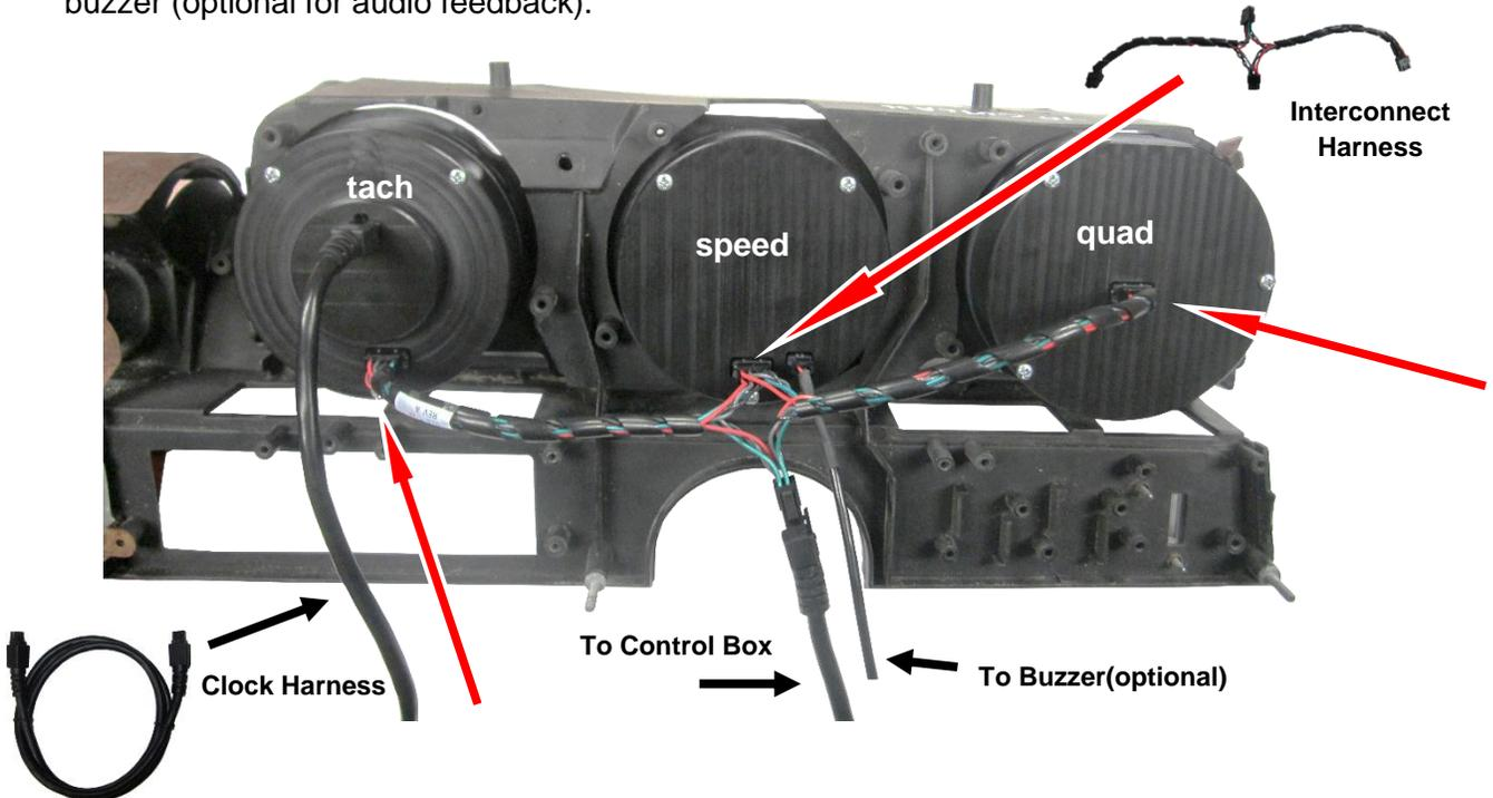
4. Re-install the gauge bezel to the dash housing using the factory hardware and refer to the main manual for wiring instructions to complete the RTX installation.
