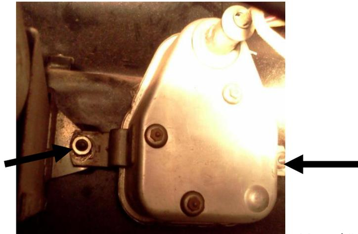
2. With the original clock removed, carefully maneuver the VLK or VLC clock in place from behind the dash while lining up the mounting holes of the clock to the studs behind the dash making sure not to scratch the chrome bezel or clear lens, and then secure the clock in place by using the stock mounting nuts.
