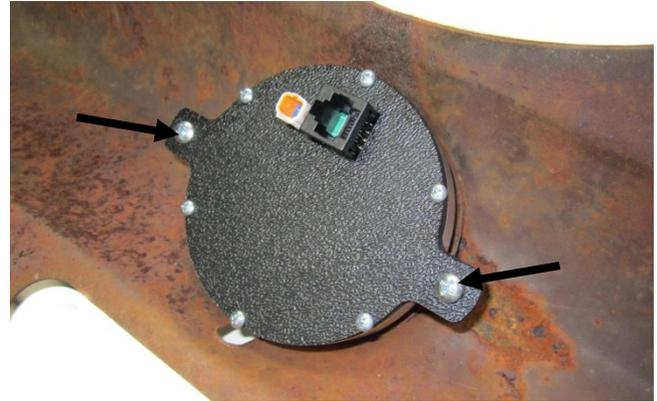
3. Connect the CAT5 cable and switch harness or VLC power harness to the clock and carefully route these back to the VHX control box and refer to the Operating Manual to complete the VHX clock setup.
