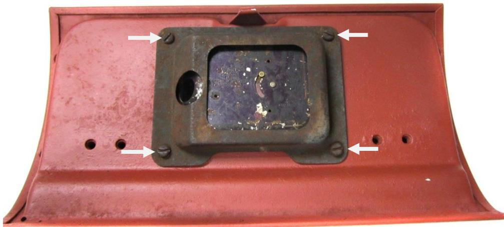
2. Remove the clock assembly and rear housing.
