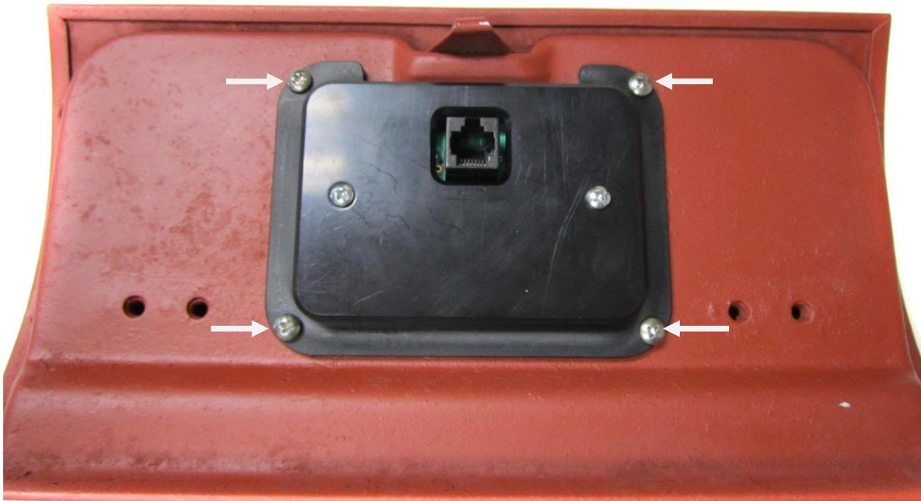
4. Connect the CAT5 cable to the new clock; with the VLC, connect the power harness as well. Take care when routing this cable to the control box.
