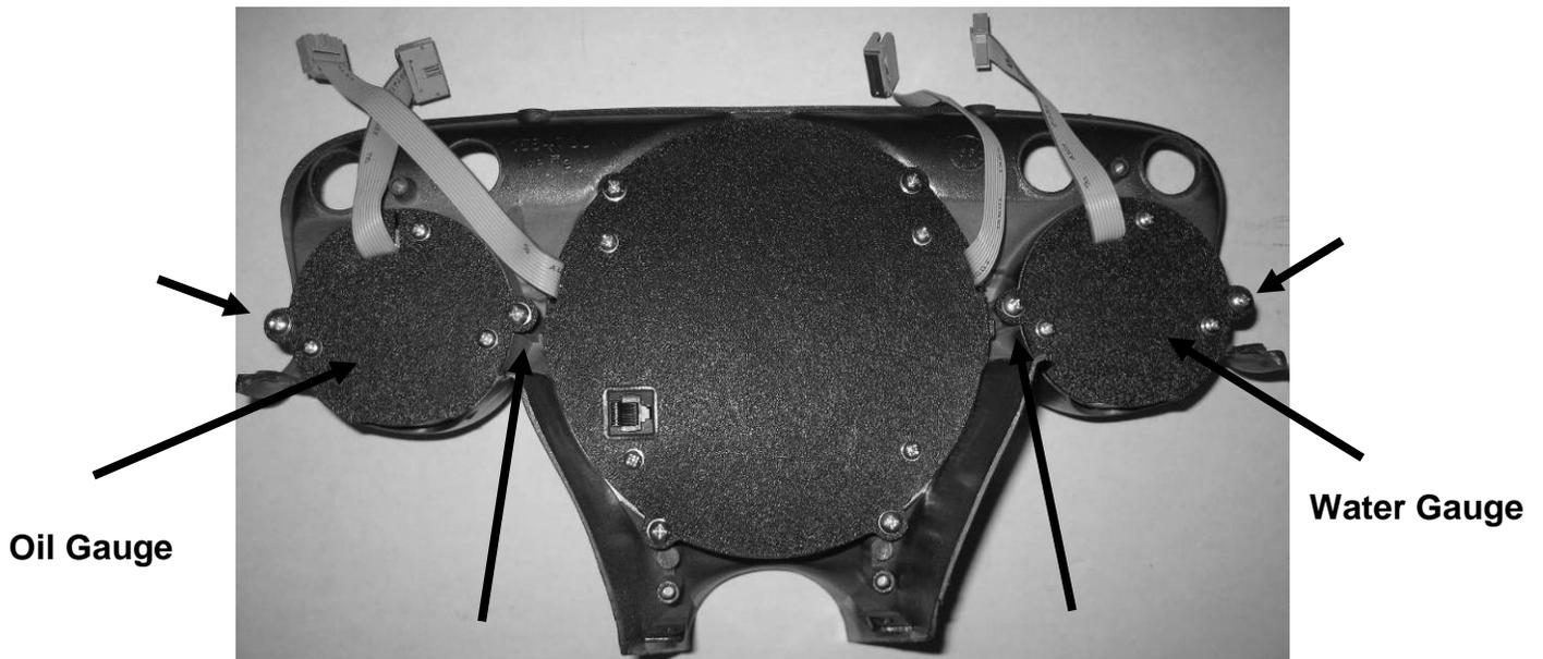
4. Connect the two smaller gauges to the center gauge via the ribbon cable connectors. These connectors are designed to plug in one way to prevent confusion.
