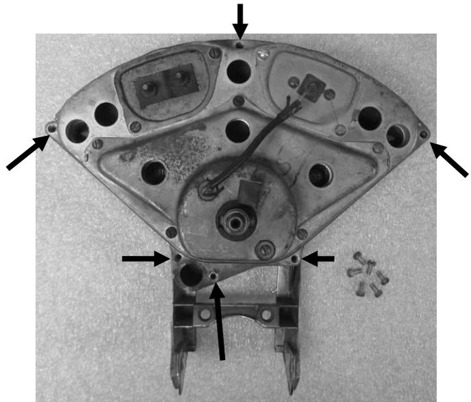
3. Remove the stock gauges, separator plate, and lens from the bezel.
