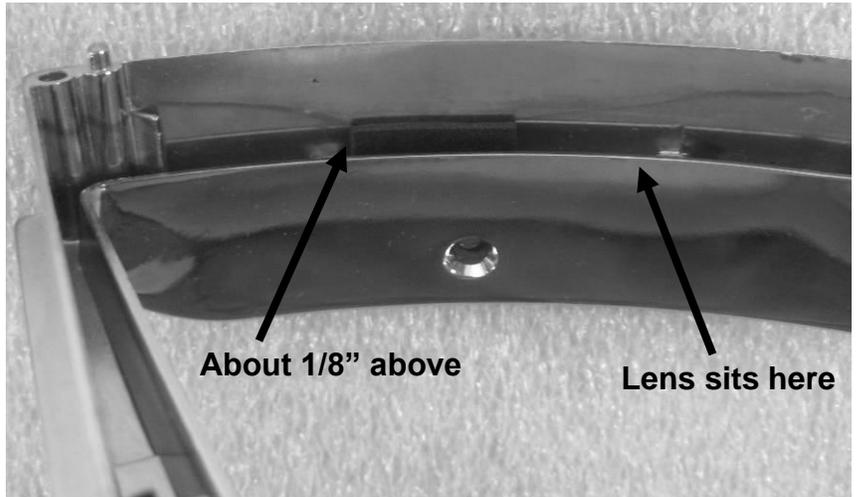
Remove the protective tape from the clear lens and install the VHX system into the bezel. Watch carefully as you insert the system so you don't scratch or damage the lens. The VHX system should align tightly with the bezel and the lens should fit flush with the bezel.
