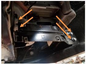
3. Remove the 2 bolts on each side that attach the bumper. Use a 15mm socket.
