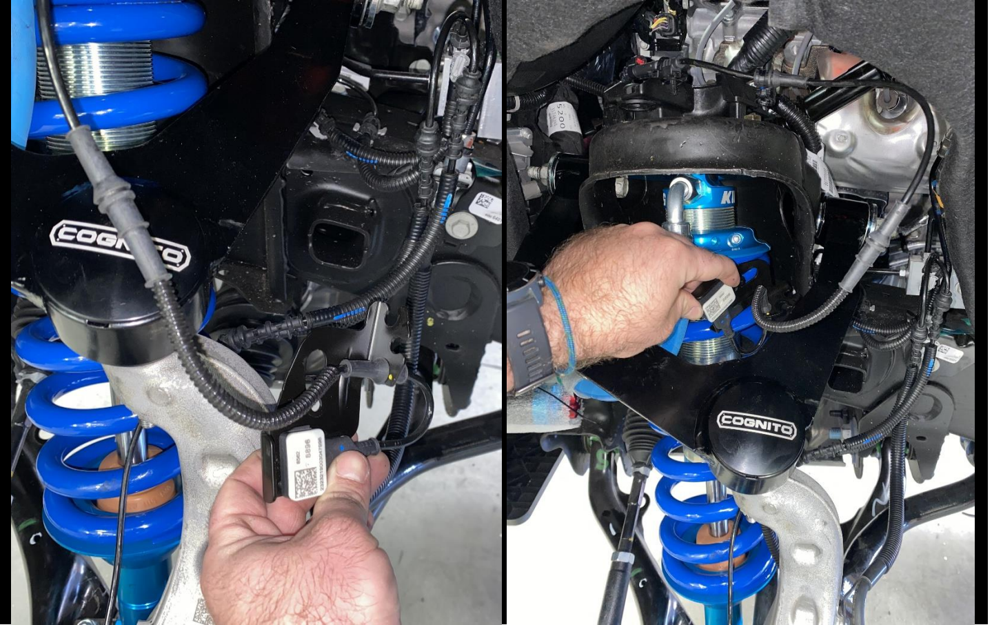
Figure 9: Remove wire bracket from spindle. Remove wires and pass bracket between arm and shock tower.
