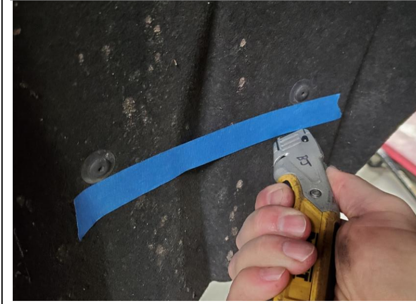
Figure 2: Cut Fender Liner Along Tape
