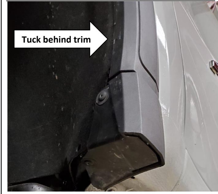
Figure 10: Plastic Mud Flap Trimmed and Reinstalled GMC
