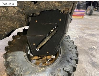
D. Locate the passenger side guard (engraved on bottom of guard XMR-22-RR) and four supplied 1/-20 x 1-1/4" flat head socket cap screw. Insert one screw through each of the four pre-drilled holes in the aarm guard through the extruded nut. See Picture 4. Loosely tighten. Once all four screws have been started tighten all fasteners securely. Repeat this for the opposite side.
