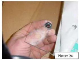
B. Insert supplied rubber grommets into the pre-drilled holes. See picture 2a. Properly installed, the grommets' shoulder edges are uniform on both sides of the windshield. See picture 2b.
