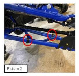
C. Once Place the Driver side a-arm guard (HTRFLV-DF) on the Driver side a-arm. Then when aligned place (2) M6 x 40mm bolts and (2) bowl washers in the locations shown in (Picture 3). Loosely tighten.
