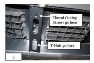
B. Using one of the supplied ¼ - 20 thread cutting screws, chase each of the pre-drilled hole by installing and removing the thread cutting screws.
