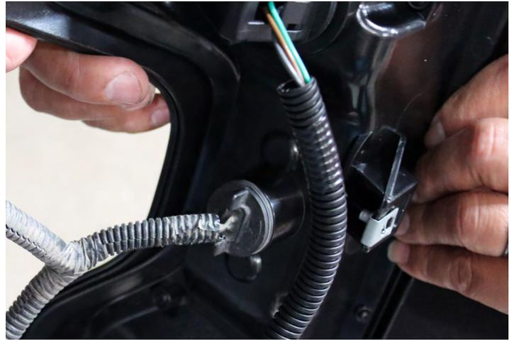
Lastly, plug the vehicle's tail light socket to new ALPHARE tail light connector.
