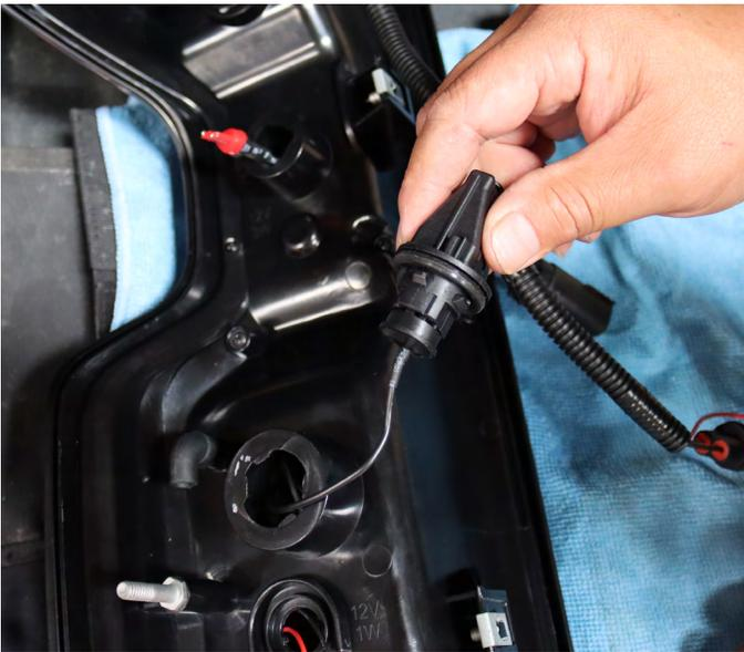
**Twist and secure the socket tightly**
