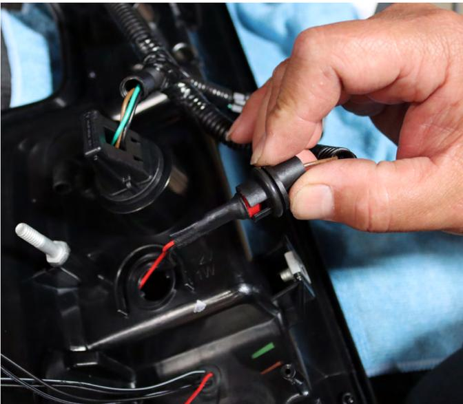
**Twist and secure the socket tightly**
