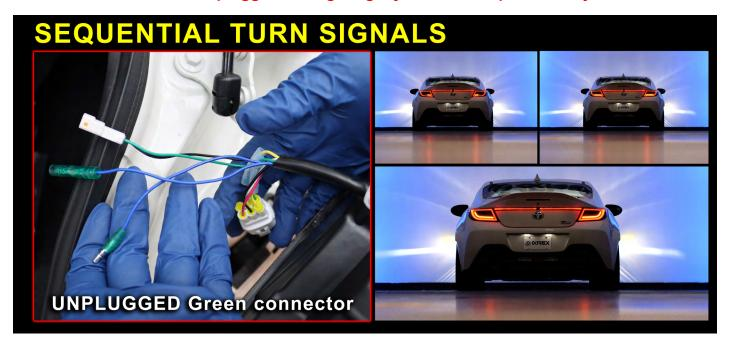
if Green connectors are connected: the lighting style will be Blinking only.
