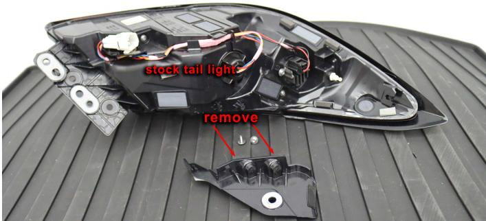
Utilize the previously removed bracket to transfer and securely install it onto the new ALPHAREX tail light. Kindly replicate the identical steps for the opposite side of the tail light.
