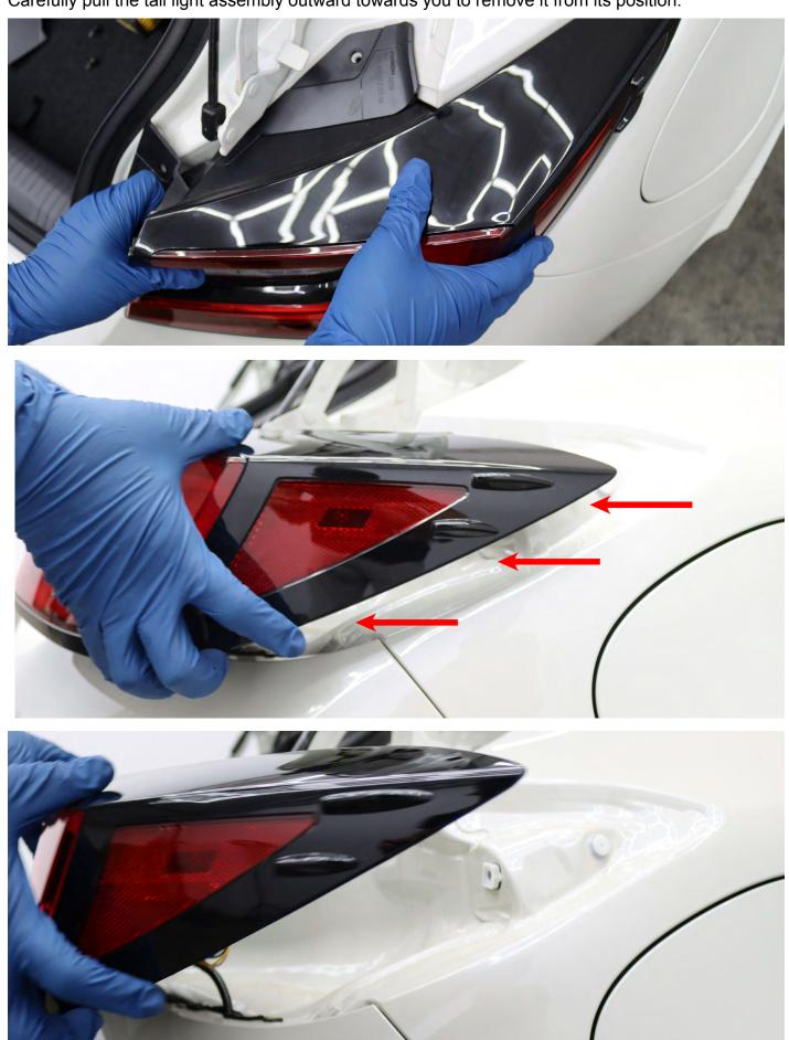
Remove the tail light by disconnecting the plug socket.
