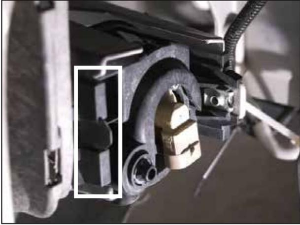
Push in the (2) tabs near the location identified above and carefully pull the fog light backwards.
