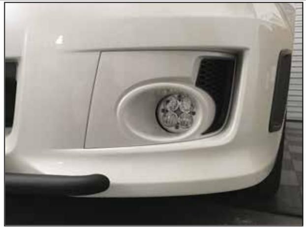
Re-attach fog cover and adjust light positioning as necessary. Wire the lights and re-attach the side vent covers.
