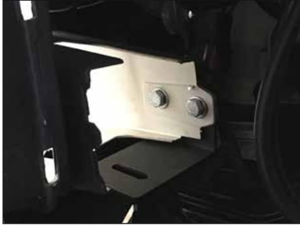
Attach the Mounting Bracket with (2) 5/16" Hex Bolts, (4) Flat Washers, (2) Lock Washers, and (2) Hex Nuts. Note that the slotted flange is on the bottom side.
