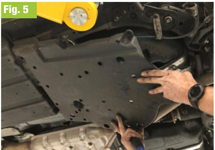
6. Support the rear sub-frame assembly with a Transmission jack or similar. (ensure you have clearance from the exhaust system).
