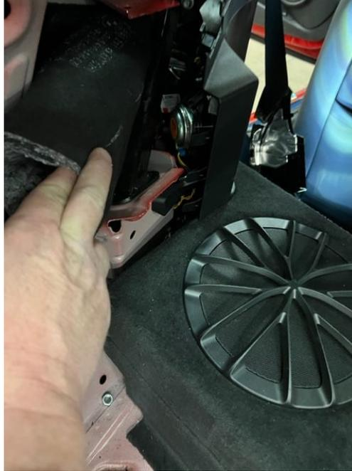
Remove the aluminum crossbar ( one T50 torx bolt on each side ) and also remove the support brackets (black aluminum rectangle tubes that run from the backside of the upper seatbelt mount down to chassis). A T12 torx bit will be needed.
