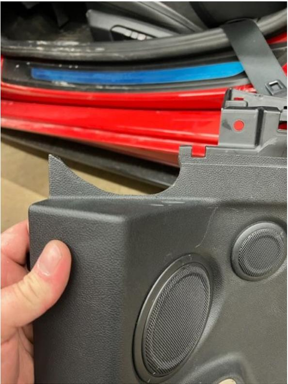
Remove the kicker plates to reinstall the trim and place the large side pieces back in their location (then re-install your kicker plates leaving the bolts loose ). Tighten all interlocking bolts to 30ft/lbs, then tighten all 10 of the mounting bolts to 50ft/lbs.
