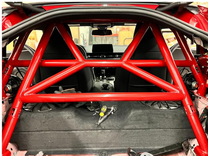
Time to start fine-tuning the interior trim. Mark out the  $\frac{3}{8}$ " holes that need to be drilled on the large side panel pieces for kicker placement.
