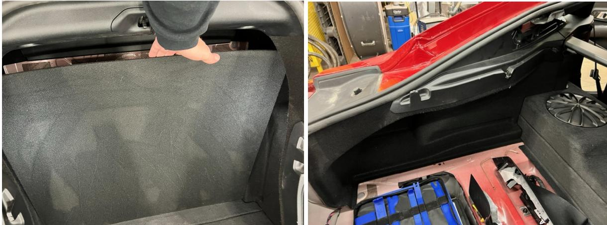
Now remove the rear trunk panel ( two T30 torx screws as well as two push pins)
