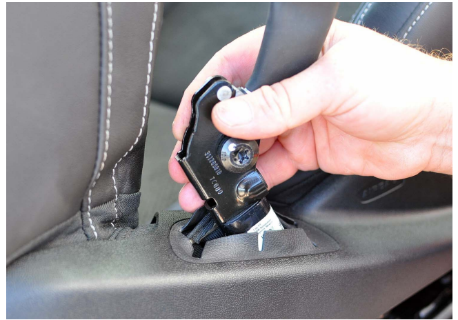
Photo E (slide airbag module up through seat, 3 pics)
