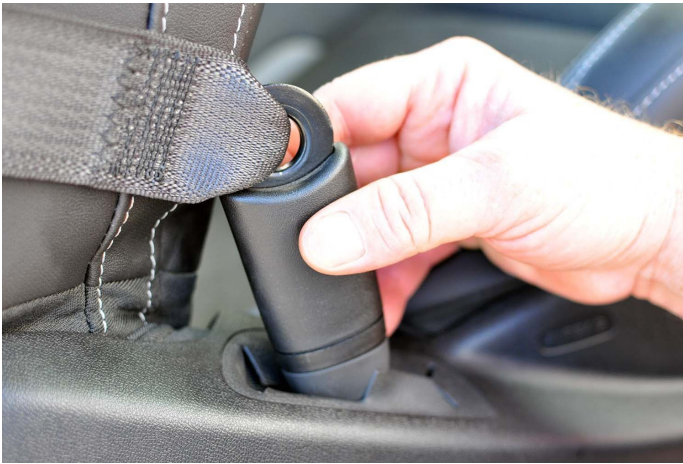
Photo E (slide airbag module up through seat, 3 pics)
