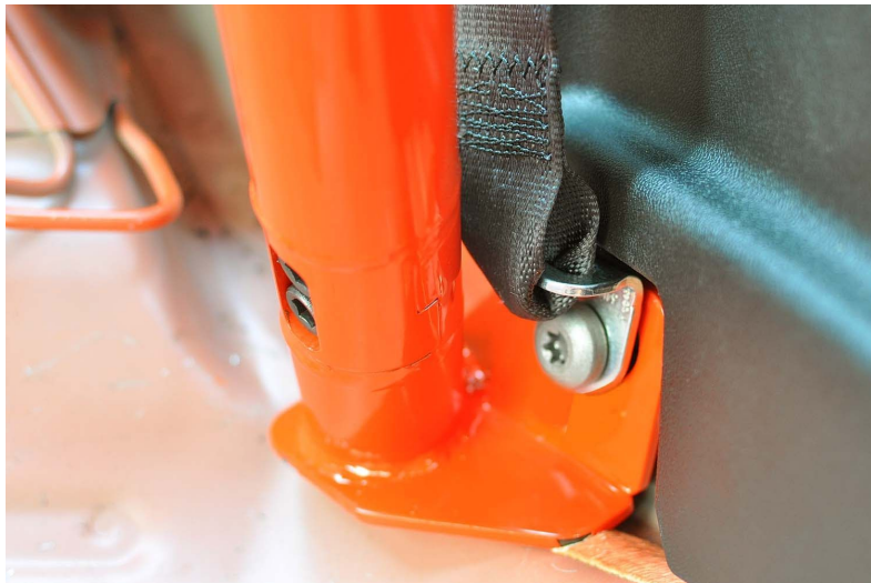
Photo M (seat belt anchor bolt thru kicker foot)
