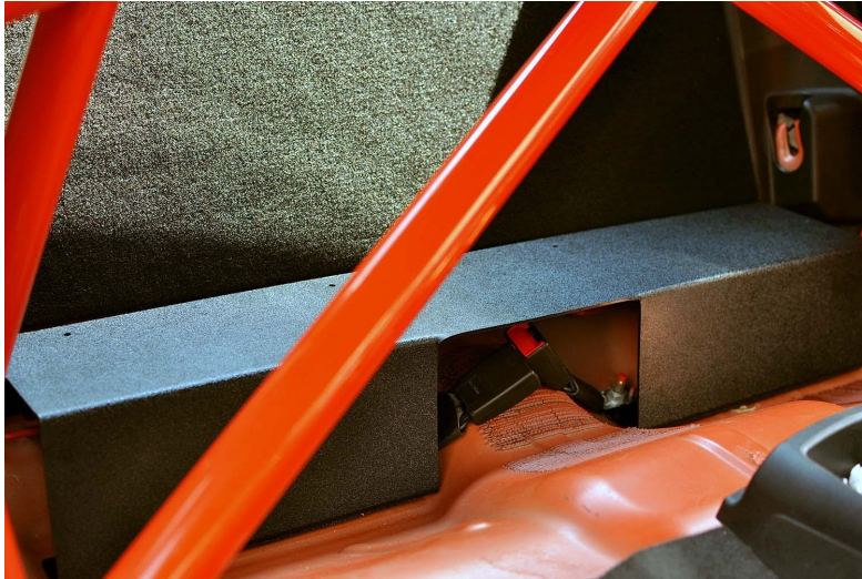
Photo P (rear seat delete lower support)
