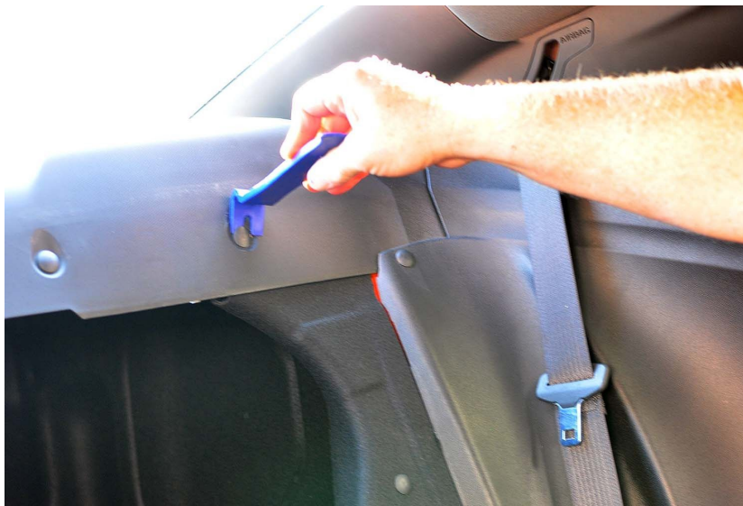
Photo G (remove rear trim fasteners)
