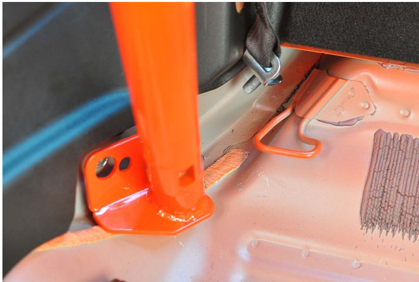
Photo K (Place roll bar with kicker lined up to feet)
