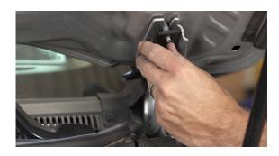
6. Take the ditch mount from above the hood and slide the end with the slotted holes under the hood and towards the hood studs. Slide the slotted holes over the hinge and hood and onto the hood studs, then put your factor nuts back on and leave snug.
