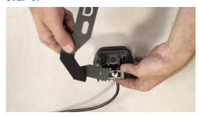
4.Attach the pod the ditch bracket. Pay attention to your pods and brackets. Some LED pods are driver and passenger side dependent, so are the ditch mounts, so make sure they are on the correct bracket. The ditch brackets have a "D" and "P" marking for driver and passenger. Using the hardware supplied with your ditch mount, put the bolt through, then attach your lock nut. Tighten snug, but loose enough to adjust later.
