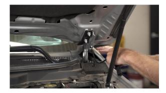
8. Route the wire down and to the position where it will be connected. You will be able to route it under rubber and plastic for a clearer more organized looking installation. 9. Close the hood slowly and check for clearance or contact. If installed correctly, the mount will not contact anything.
