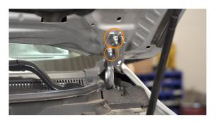
5. Pick a side, drivers or passenger and grab the ditch mount and LED that go to that side. Using a wrench or socket, remove the nuts that attach the hood to the hinge, there will be two nuts on each side. Remove the nuts and hold the hood in place so that the hood does not dip down and get damaged.
