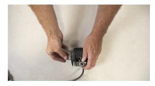
3. Assemble your LED pod. Depending on which LED pod you get, there are different brackets and ways to attach them. Got the brackets on the pod and leave semi loose for adjustment later.
