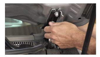
Then tighten the two factory nuts down to the factory torque spec for year and model.
