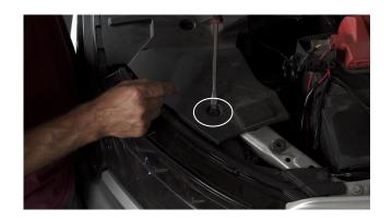
Remove the two 8mm bolts that hold the intake scoop in place.
