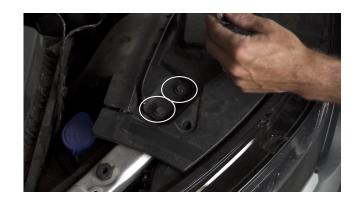
Remove the 2 screws that hold the grill to the body.
