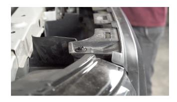
Remove the 4 torques screws that hold the inner air deflector in place.
