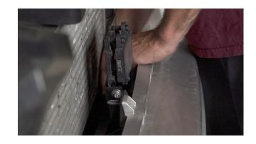
Plug in the connector in the back, then follow Ford's radar leveling and locating procedures.
