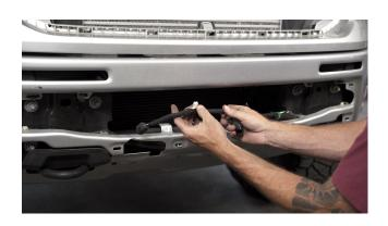
Now install your radar to the truck. Grab an included bolt and install a washer. Then put a washer on the bottom, and finally the lock nut. Get the bolts on both sides, adjust your radar to the desired position and tighten the bolts.
