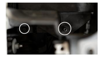
Remove the air deflector, push down on the front an lift the back while pulling it forward, it will slide down and then be able to be removed through the top.
