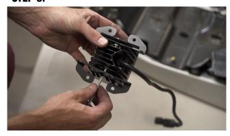
Now we will install the brackets to the pods. They brackets are universal for position, so light up the bracket and install the pod hardware. Leave loose. Put the pod into position on the truck. Put the 4 torques bolts back in and tighten down.
