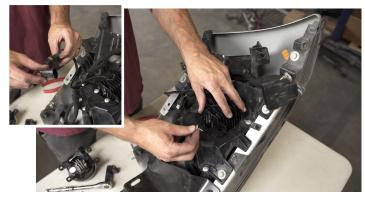
Then using the LED wrench, push the pod flush against the plastic of the bumper and tighten in place. Check the front for straightness. Using the adapter plug, connect the LED pod and the factory harness.
