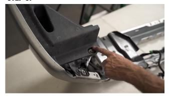
With the bumper on a table or work bench, remove the plastic trim. There are 2 bolts to remove with an 8mm and a black plastic clip on top.
