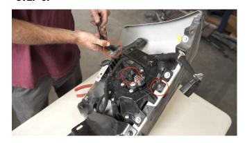
Next there are 3 bolts that hold the factory fog light cover to the truck. Remove the 3 bolts and set the bracket out of the way.
