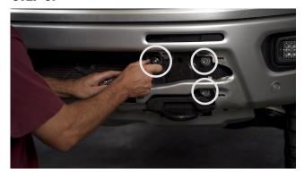
Remove the nuts that hold the bumper to the frame, there will be three nuts on each side to remove with your 21mm socket. Be cautious the bumper can fall off, hold in place.
