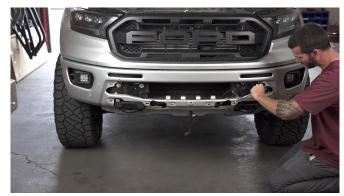
With a friend reinstall the bumper, ensuring to plug in the big plug on the drivers side. Put the bumper on a loosely install the bumper nuts. Then with a friend lift the bumper up tight against the grill and fenders and tighten the nuts. Make sure level before tightening in place. Re-install the remaining bolts, trim pieces and fasteners. Refer to the direction above.
