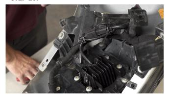
Wrap up any excess wiring and lip tie out of the way.
