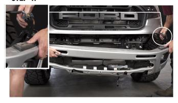
With the help of a friend pull the bumper away from the truck. On the drivers side near the tire there will be a large wiring connector, unplug this before completely removing the bumper.
