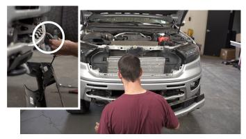
Remove the trim panel. This is held on by tension clips. You will have to work your way around pulling on the panel and remove it from the bumper. Unplug the parking sensor harness. If you have factory mud flaps, remove the silver bolts in the bottom corner of your front wheel well with an 8mm. Reach in the opening and unplug the wiring connector you see on drivers side.
