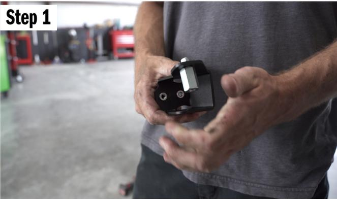
Get your  $\frac{1}{4}$  bolt, split lock washer and flat washer. Put the lock washer on the bolt, then the flat washer. Then put the bolt through the mount. Then thread on the hex stand off. Tighten all the way with your allen tool and wrench.
