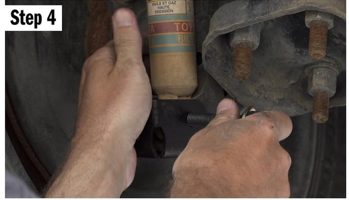
Take the shock skid and put the hex standoff in the  $\frac{3}{4}$ " hole behind the shock. Then rotate the shock skid up and in position.
