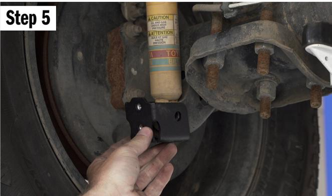
Take the new shock bolt supplied with the hardware kit and put on a washer. Then put it through the shock skid and shock mount. You may need to use a screw driver or alignment tool in order to get the shock in position and line up the bolt. This can be tricky to align, but it will come together when lined up. Once the bolt goes through, put on the other washer and the lock nut.
