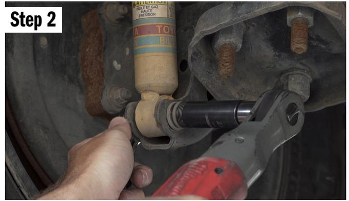
Remove the factory shock bolt with a 17mm socket and wrench.
