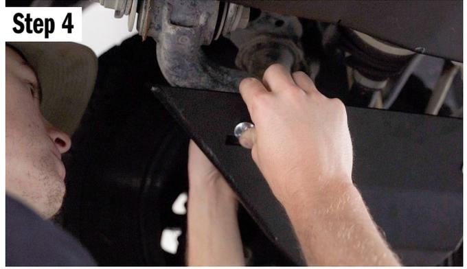
Using the longer 3/8 carriage bolt, place it into position towards the rear of the skid plate. Push it through the lower control arm and put on a washer and a nut. Hand tighten.
