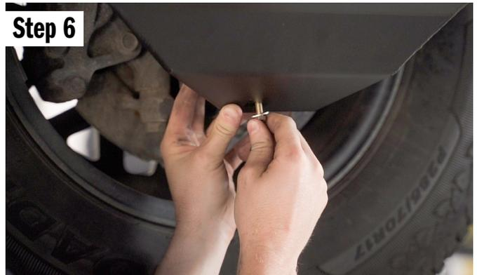
Use the 1/4" bolt, add a washer, push the bolt through the skid and through the aluminum spacer. Note: Only the 2nd Gen Tacoma will require the aluminum spacer.
