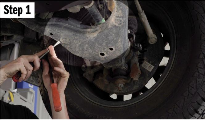
First you will need to remove the plastic caps that are located on the lower control arm. Use can use a flat screwdriver or pry bar to remove them.
