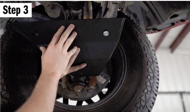
Using the shorter 3/8 carriage bolt, place it into position towards the front of the skid plate. Push it through the lower control arm and put on a washer and a nut. Hand tighten.
