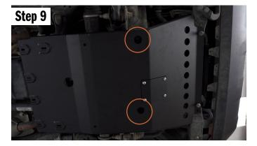
Starting with the (2) 17MM bolts in the center, tighten them until tight. The skid plate will suck up into position. Then tighten the (3) bolts in the front, then the (2) 13mm bolts in the rear.
