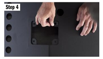
Then, add the oil filter door to the skid plate by sliding on the clip on nuts over the tabs inside the oil filter doorway. Be sure to align the holes to allow for the bolts to install easily.
