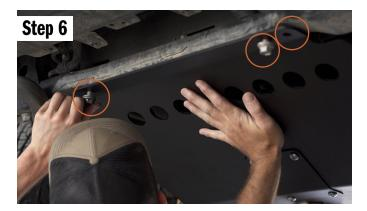
With a floor jack or friend lift the skid plate in place. Starting at the very front, install the factory bolts you just removed in all (3) locations. Leave these loose
