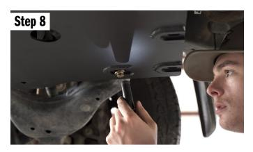
Use an M8 bolt, put on a split lock washer, and a flat washer, and thread them into the holes. Put these in snug, DO NOT TIGHTEN.
