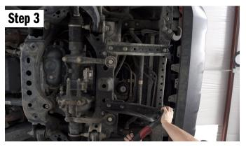
With the factory skid removed, we now need to remove the factory front supports. Using a 17MM socket, remove the (7) bolts.
