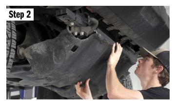
It is recommended to move the front bolts, then remove the back bolts to allow the hooks to catch and swing forward the skid. Once both plates have been removed, set them aside and hang onto the hardware.
