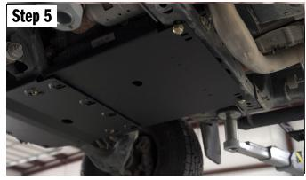
Next install the (4) 3/8's bolts into the holes. These should fit flush to the frame.
