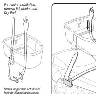
Thread Pronghorn Strap, small end down, through the slot on the bottom of Klamath. Slide on two fender hooks, facing each other as shown. Position Klamath as desired, secure hooks on either side of fender. Repeat for second strap
