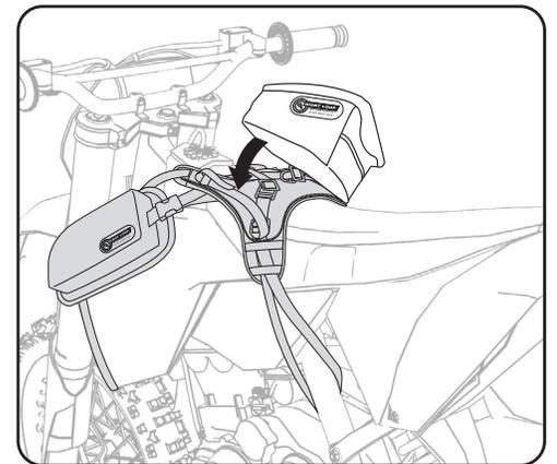
**3** The Tank Bag is designed to allow easy access to your fuel filler by simply unzipping one side of the bag from the harness. Note that the concave shape of the Tank Bag's front allows vent tubes to breath. Unzip the Tank Bag on both sides to remove it from the harness and take it with you, leaving the harness mounted and ready to go.
