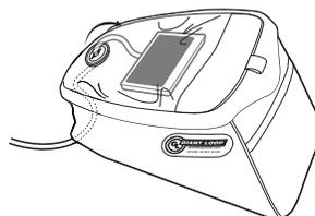
**C** Reach into mesh pocket to pass power cable through rubber grommet to power devices in top map pocket.
