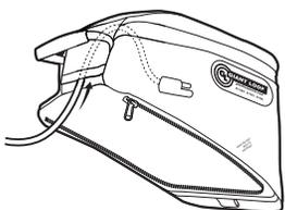
**A** Thread power cable through flap on front of Tank Bag and re-secure hook-and-loop to prevent water migration.
