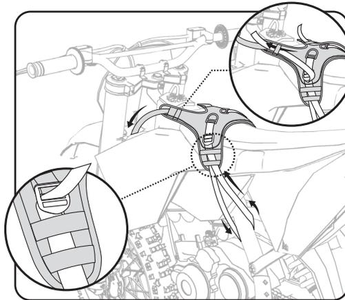
**2** Locate the appropriate connection points on each side of frame. Use the farthest forward positions available (i.e., the shortest distance). Loop each side's webbing straps **around frame/subframe** and back up through reflective tabs and thumb-lock buckles. **DO NOT** allow webbing to contact exhaust! Tighten all three points of contact and secure all loose webbing ends.
