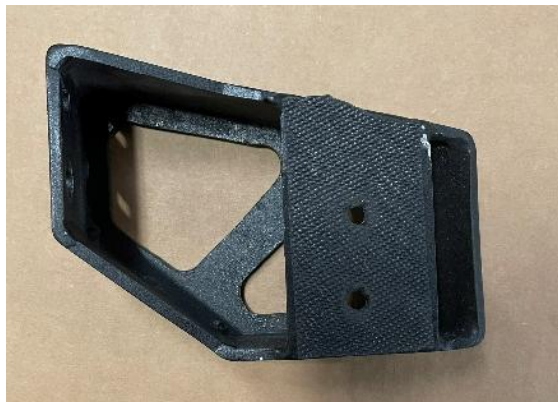
Figure 2: HD Lower Bracket with Foam Tape
