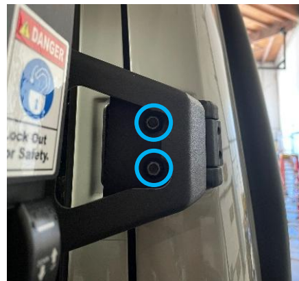
Figure 14: Heavy Duty Upper Bracket Mounting
