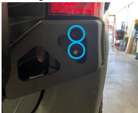
Figure 13: Heavy Duty Lower Bracket Mounting
