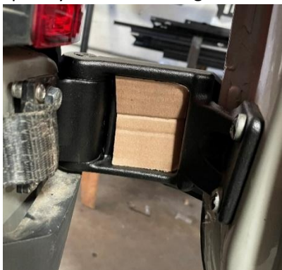
Figure 11: Cardboard to Push Bolts Out on Lower Hinge
