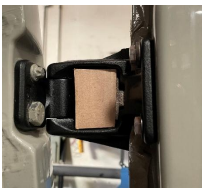
Figure 12: Cardboard to Push Bolts Out on Upper Hinge
