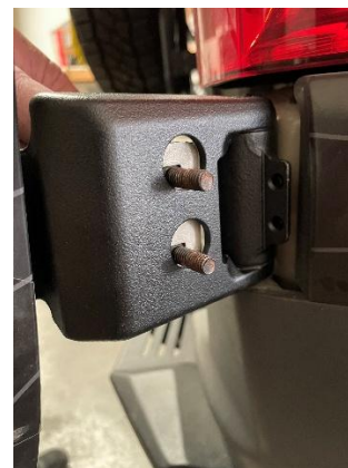
Figure 9: Lower Hinge Bolt Routing
