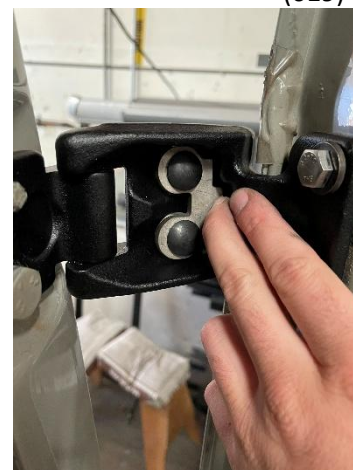
Figure 8: Upper Backing Plate Insertion
