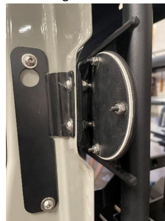
Figure 15: Base Unit Emblem Replacement Mounting
