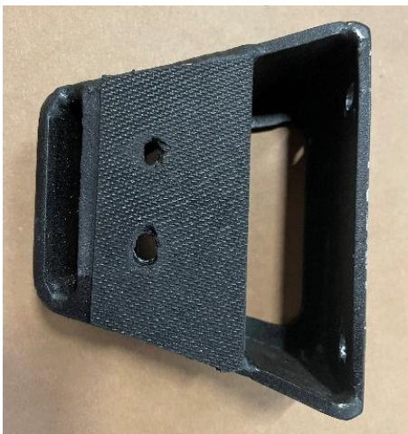
Figure 1: HD Upper Bracket with Foam Tape
