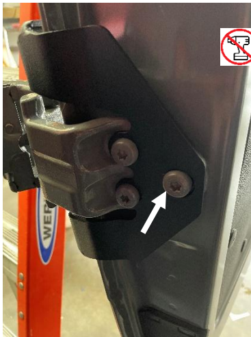
Figure 7: Bracket Installed Over Factory Hinge
