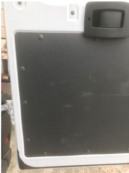
Figure 12: Remove Plastic Door Rivets
