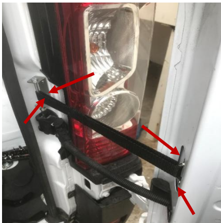
Figure 18: Completed Door Strap Installation
