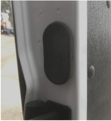
Figure 11: Remove Rubber Door Grommet
