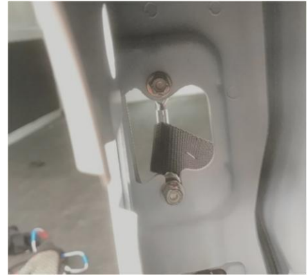
Figure 14: Backside View of Door Stop Mounting
