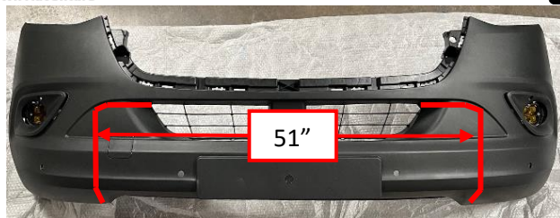
Figure 29: Marking Front Bumper Cutout
