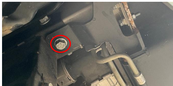
Figure 21: Installed Factory Crossmember Bolt Thru Winch Tray
