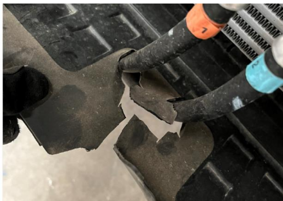
Figure 15: Air Flow Skirt Cut for Removal
