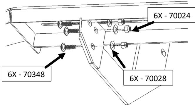
Figure 1: Bolting Mounting Blades to Nerf Step
