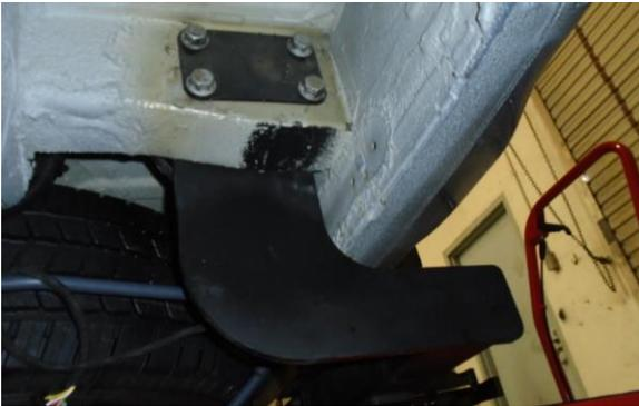
Figure 2: Four (4) of the Hitch Mounting Bolts
