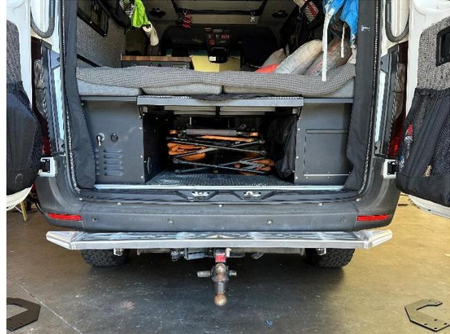
Figure 3: Hitch Clearance with Rear Nerf Step Installed
