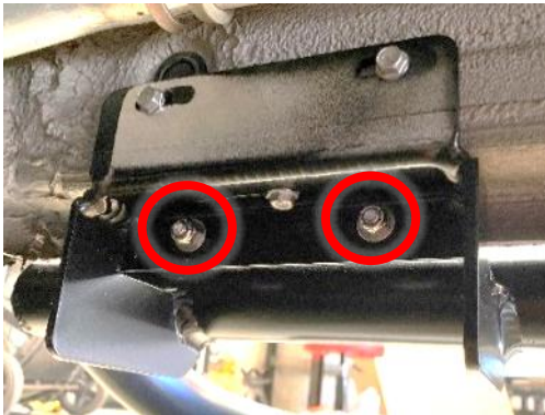
Figure 5: Pinch Weld Fastener Installation
