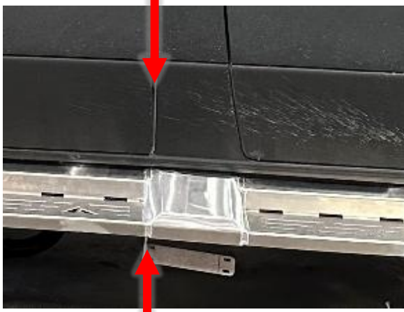
Figure 1: Side Step Alignment with B-Pillar Seam
