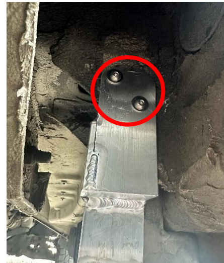
Figure 7: Rear Support Bracket Upper Mounting
