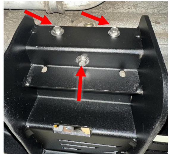
Figure 2: Step Bracket Installation Behind Pinch Weld
