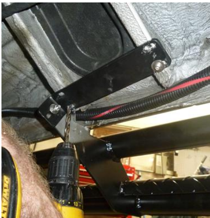
Figure 10: 90 Degree Bracket Installation onto Van
