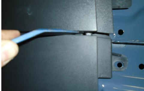
Figure 7: Removing Small Plastic Panel from Rear Bumper
