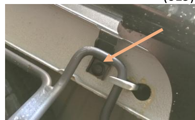
Figure 3: Plastic Rivets Underneath Bumper
