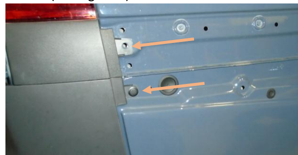
Figure 6: Plastic Rivets Underneath the Side Panel
