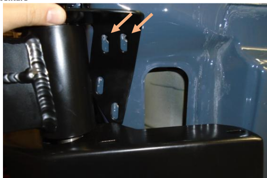
Figure 11: Drilling for Axle Support Bracket
