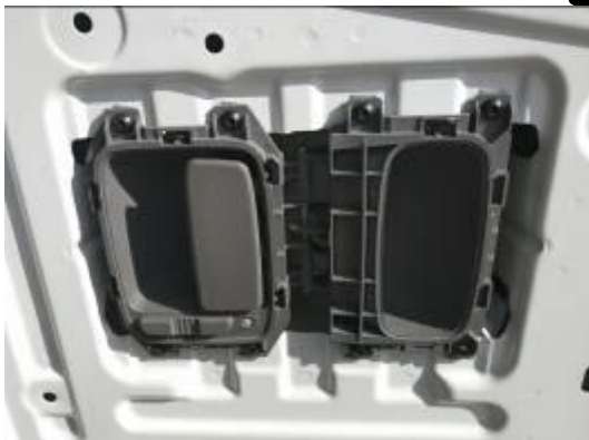
Figure 4. Torx bolts holding door handle on passenger side door.
