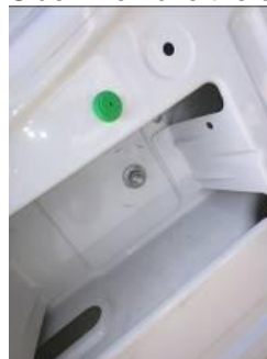
Figure 2. Door magnet bolt underneath door panels.
