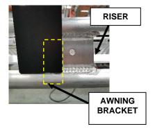
4. Drill a ¼" hole through the bottom of the bracket and into the awing. Using the supplied Fiamma hardware, bolt the brackets to the awning using one bolt on each bracket. Center the brackets to the closest riser. Set front and rear brackets as close to support sticker as possible.
