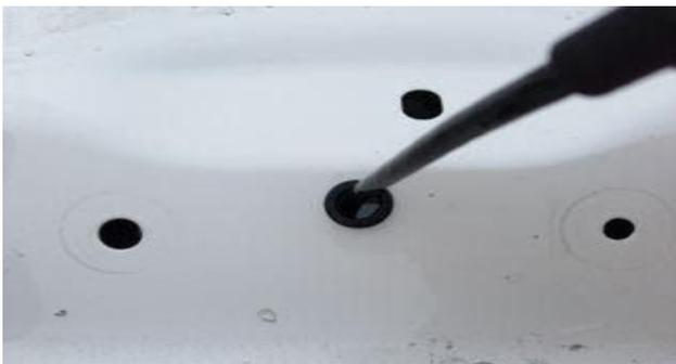
**Step 5:** Route camera and/ or chassis harness along existing wiring and secure using wire ties or electrical tape. **IMPORTANT:** Ensure harnesses move freely with the trunk or liftgate.
