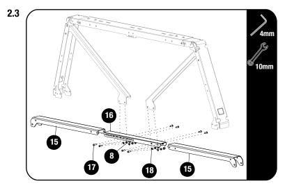
Loosely assemble the vehicle specific mounting brackets, refer to fitment guide supplied.
