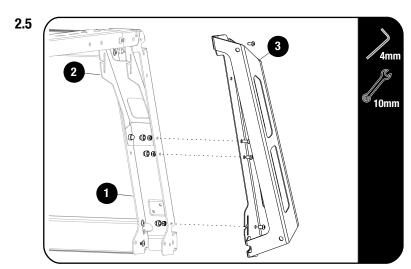
Fit the Pro Bed Rack rear Coner Bracket (Item 3) in to the Leg Sticker assembly (Item 1) Use the M6 x 12 Butto Head Bolt with the M6 Nyloc Nut (Item 7 & 8). Do not Fully Tighten.
