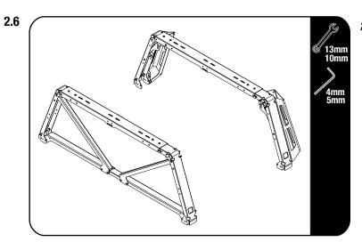
With all the brackets in place tighten all the M8 and M6 bolts and place Nut caps ehere needed.
