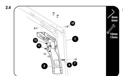
Slide the Pro Bed Rack Support Bracket (Item 2) in to the Leg (Item 1) using the M8 x 20 Button Head bolt, M8 x 19 x 2 Flat washer and M8 Nyloc Nut (Item 10,11&12)
