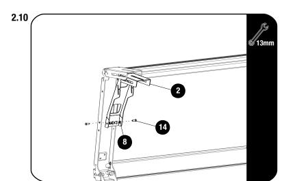
Loosely assemble the M6 x 12 Button Head bolts, M6 x 12 x 1 Flat Washers and M6 Nyloc nuts (Item 2 , 4 & 18).D0 NOT FULLY TIGHTEN.
