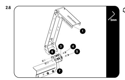
Assemble the Pro Bed Leg (Item 1) on page 3 to the bracket fitted in 2.1 using M8 x 25 Button head bolts, M8 x 19 x 3 Flat washers and nyloc nuts (Item 3,5 & 7) as shown and M8 x 20 Button head bolts and M8 nyloc nuts (Item 4 & 6).
