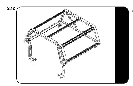
Fully Tighten all the bolts and nuts and place nut caps where needed.
