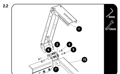
Assemble the Pro Bed Leg (Item 1) on page 3 and the Front Horizontal Support Bracket (Item 15) to the bracket fitted in 2.1 using M8 x 25 Button head bolts, M8 x 19 x 3 Flat washers and nyloc nuts (Item 3,5 & 7) as shown and M8 x 20 Button head bolts and M8 nyloc nuts (Item 4 & 6).
