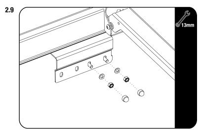
With the Load Bed Rack in position fully tighten the bracket fitted in 2.1 & 2.5.
