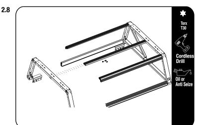
Pull the Front assembly with the extrusion toward the rear legs.
