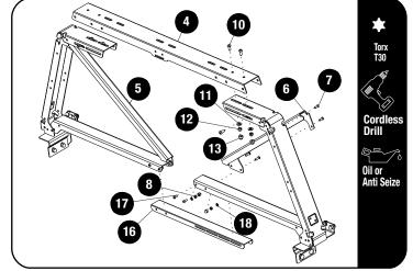
Assemble the Front diagonal and Horizontal Brace parts as shown (Item 4, 5 & 6) to the legs fitted in 2.2 using the M8 x 20 Button head bolts M8 x 19 x 2 flat washer and M8 nyloc nuts (Item 10 , 11 & 12).
