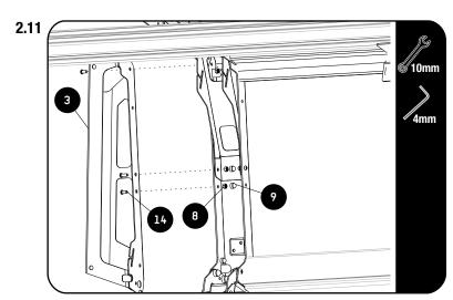
Assemble the Rear Wing Brackets (Item 3) to the back of the frame using the M6 x 12 button head screws, M6 x 12 x 1 Flat washers and M6 Nyloc nuts (Item 14, 8 & 18).
