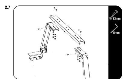
Loosely assemble the Cross Brace to the leg assembly using the M8 x 20 Button head screws, M8 x 19 x 2 Flat washers and M8 Nyloc Nuts (Item 10 , 10 & 12). Fully Tighten the M8 Button Heads.
