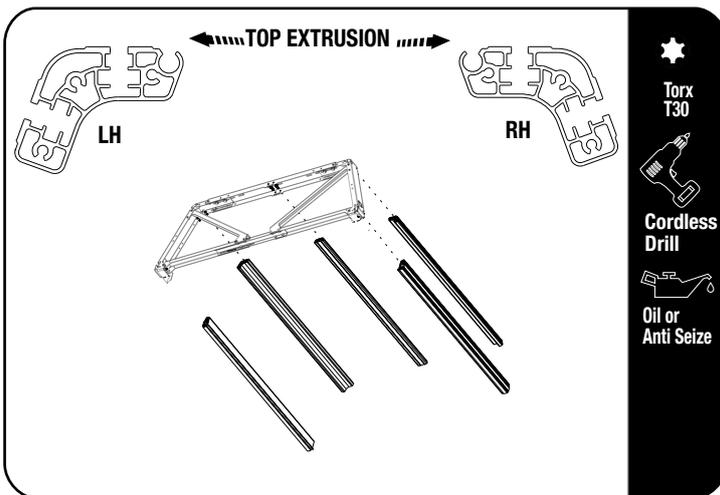
Slide the front leg and truss assembly backward to allow access for securing the extrusions.
