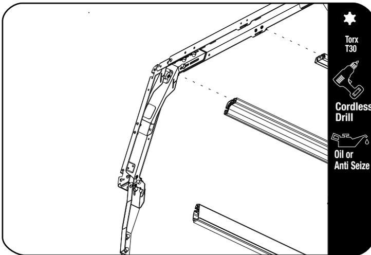
⌚ Pull the front leg / truss / extrusion assembly toward the rear legs. Attach the rear leg assembly to the Extrusions using the M6x25 Thread Forming Screws (Item 19) and a cordless driver. The front assembly will be pulled back into its final position while fully tightening these screws.
