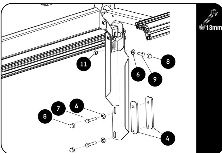
With the help of a friend, lift the Pro bed Rack on to the load bin and loosely fit the M8 x 45 and M8 x 19 x 2 Flat Washer into the OEM mounting points together with the 10mm large spacer (Item 7, 6 & 4). **DO NOT FULLY TIGHTEN.**
