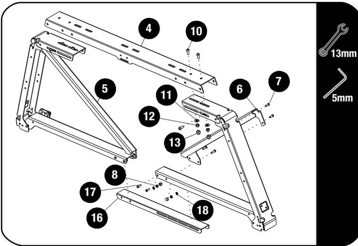
Assemble the Front Diagonal and Horizontal Brace parts as shown (Item 4, 5 & 6) to the legs fitted in 2.2 using the 8 x M8 x 20 Button Head Bolts, 8 x M8 x 19 x 2 Flat Washer and 8 x M8 Nyloc Nuts (Item 10, 11 & 12).
